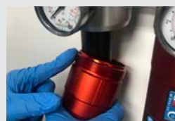
4. Grease and place lower section
