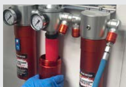
1. Unscrew lower section
