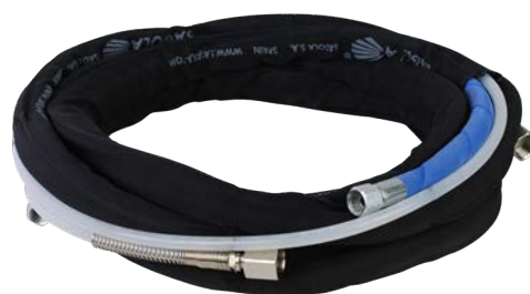
Air and product hose set for low-pressure equipment. 8 x 15 mm. anti-static air hose and 6 x 8 mm. product hose with Nylon cover. Light and resistant hose. (see page 161)
