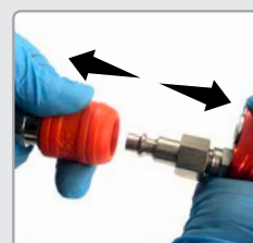
4. Disconnect the plug
