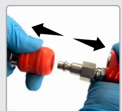
4. Disconnect the plug
