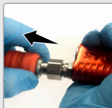
2. Pull the body as the arrow indicates
