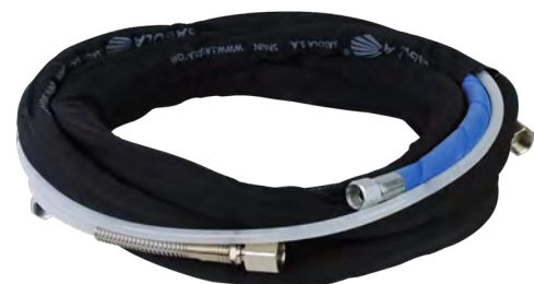
Air and product hose set for low pressure equipment. 8 x 15 mm. anti-static air hose and 6 x 8 mm. product hose with Nylon cover. Light and resistant hose. (see page 147)
