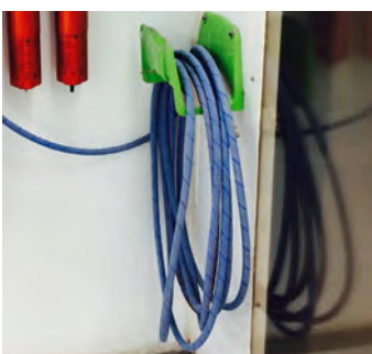
Heated hose system. Independent of ambient temperature.
